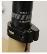
We must use a torque wrench, using the tightening marked on the stem in newtons/meters, respecting the maximum and minimum indicated on the part itself. If you need a height greater than the minimum insertion mark [Photo 2], it would be convenient to check that the size chosen is correct. For the rest of the seat adjustments (inclination, forward/backward...), you should contact the manufacturer of the seat to obtain its user manual.
